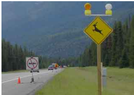
Figure 6.37: Deer crossing sign with flashing lights (Friedman, 2005)
